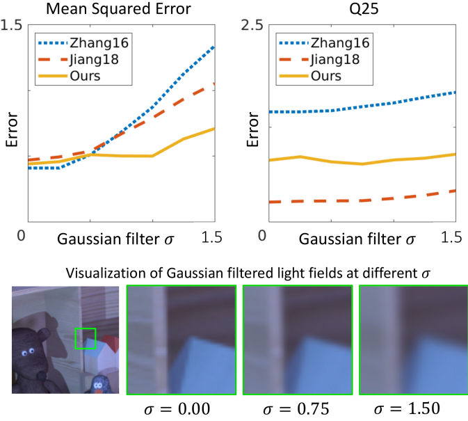
Figure 13: Robustness of our method to low-gradient edges ( Dino light field; we compare to the methods of Zhang et al. [25] and Jiang et al. [18] which have the best MSE and Q25 performance on this light field, respectively).
