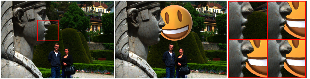
Figure 20: Additional light field editing result. Left : input scene. Center : Our editing results. Right, clockwise from top-left : Detail of the unmodified light field image, Zhang et al. [16]’s editing result, Shi et al. [19]’s editing result, and our result with fewer artifacts.
