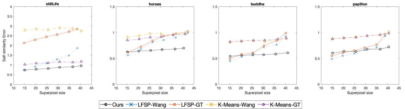
Figure 10: Self-similarity error measured over all light fields in the HCI dataset. This error provides a measure of the consistency of superpixel shape across views; smaller errors indicate greater consistency.
