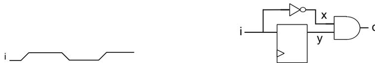
The circuit indicates the functional relationship between signals  $i$ ,  $y$ , and  $x$ ; the timing diagram for  $i$  can be extended to reflect these relationships; the resulting diagram appears below on the left. Given the waveforms for  $y$  and  $x$ , the diagram can be further extended to display information about signal  $o$  as in the diagram on the right:
