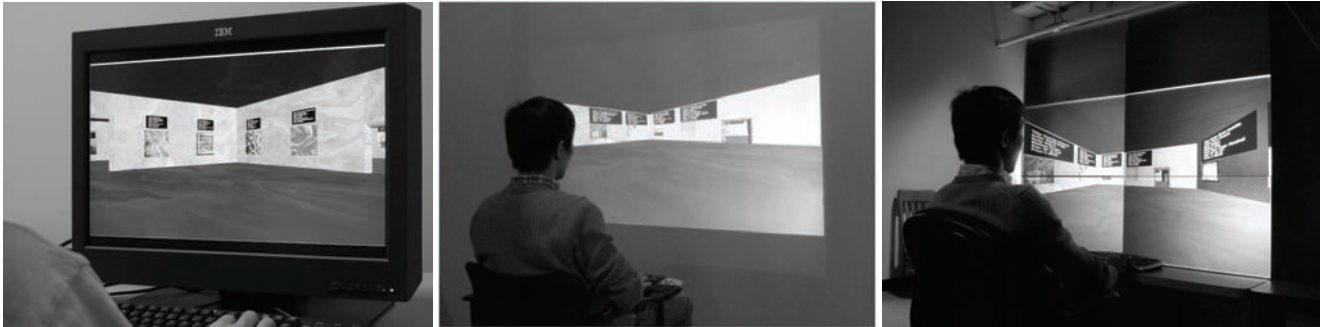
Figure 1. Apparatus used in our experiment. From left to right: (a) High-resolution IBM™ T221 LCD flat panel, (b) Rear-projected screen, and (c) VisBlocks™ tiled high-resolution display module.
