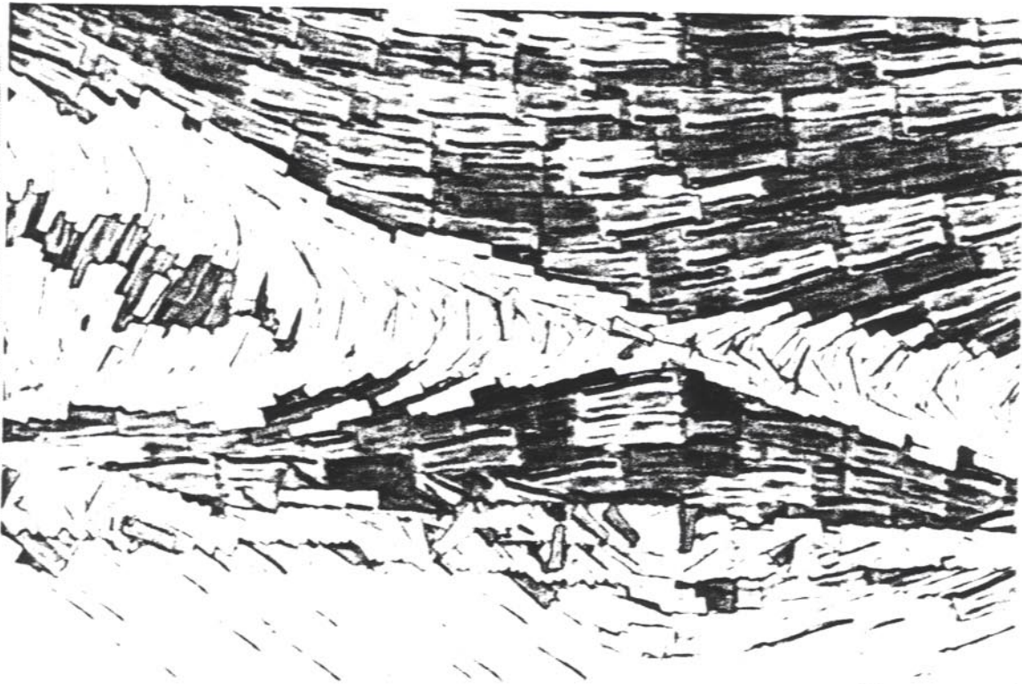
Figure 3: A preliminary example of a "painterly" visualization of the velocity of fluid flow over an airfoil. Two layers were used. The bottom layer shows the data low-pass-filtered and represented with brush strokes the size of filtered features. The texture of the strokes indicates the flow direction. The top layer shows the unfiltered data with much smaller brush strokes, which are only visible where the curvature of the velocity field is large. The stroke color also encodes the magnitude of the curvature, varying from yellow to orange. In this illustration the data is 2-D, but the techniques will also apply to volume data.
