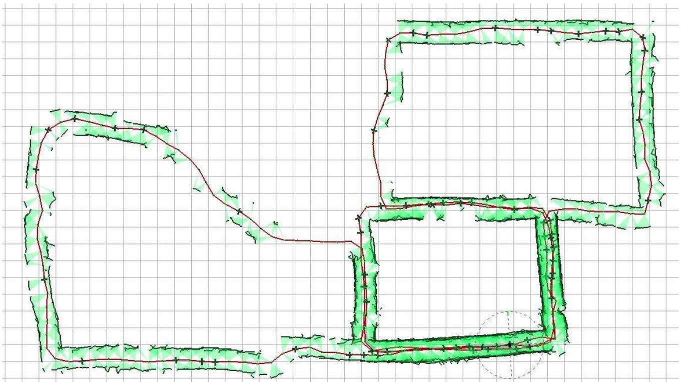
Figure 6: A 250m drive from the AI Lab. Map computed offline using 5000 particles.
