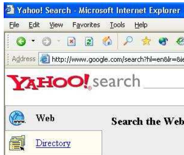
Figure 5.1: This window may look authentic, but all content below the file menu is fake. Using Javascript, one can actually even interact with the toolbar.
