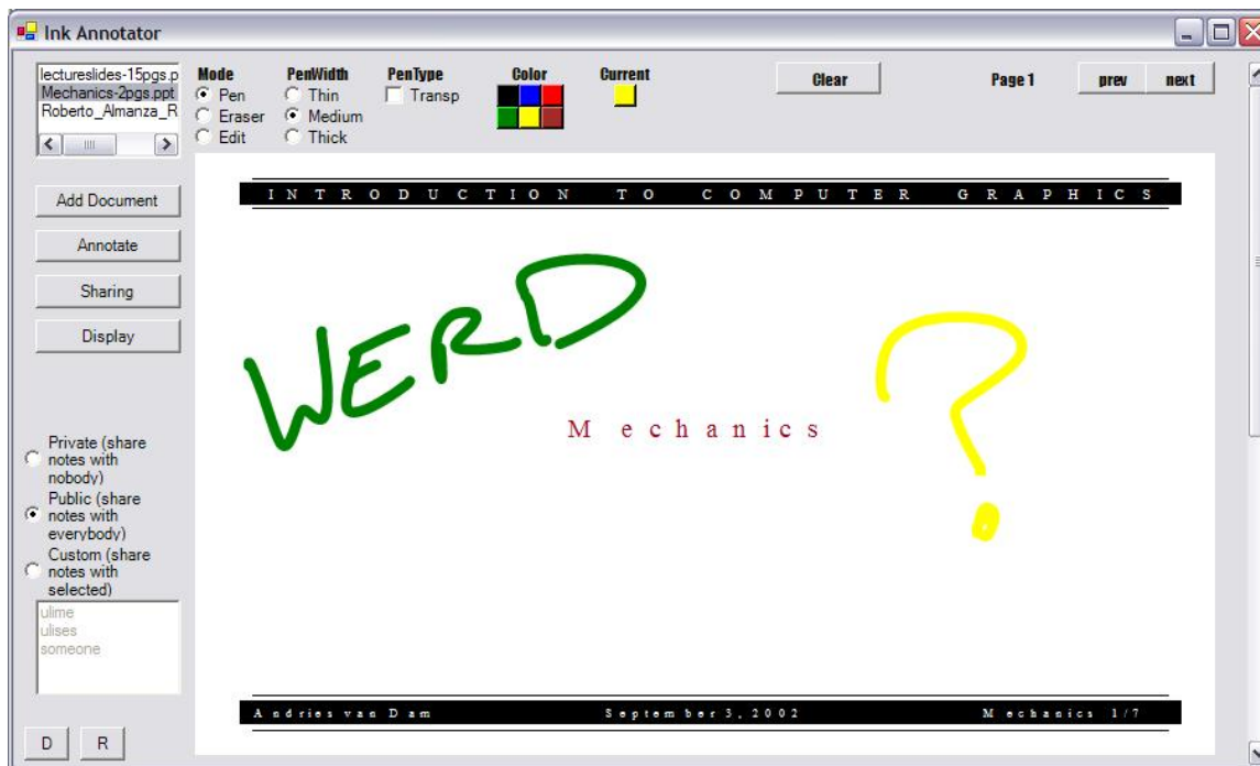
Figure 4: A screen shot of the current user interface. Documents available for annotation appear in the top left. The user can select sharing modes in the bottom left, and drawing on the current document with the stylus will result in annotations.
