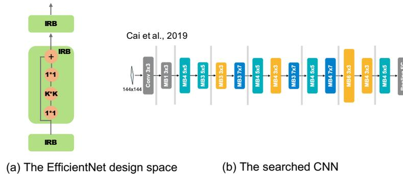
Figure 2.4: The illustration of EfficientNet search space.
