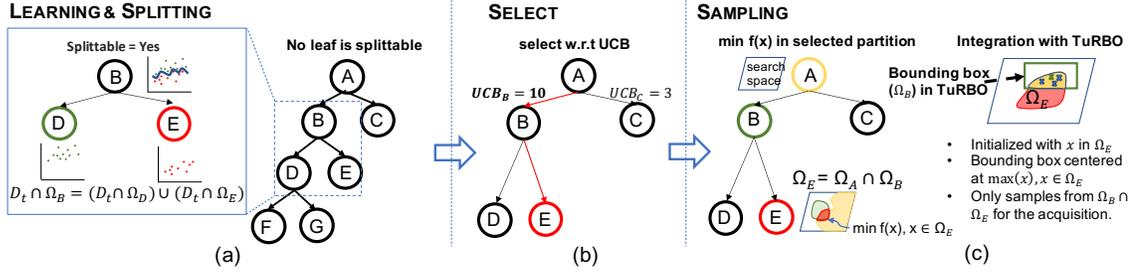
Figure 5.2: The workflow of LA-MCTS: In an iteration, LA-MCTS starts with building the tree via splitting, then it selects a region based on UCB. Finally, on the selected region, it samples by BO.
