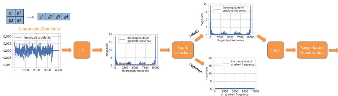
Figure 7.3: The gradient compression framework (sender).
