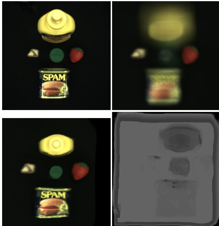
Figure 3.4: Top Left: A single image from the wrist camera, showing perspective. Top Right: Refocused image converged at table height, showing defocus on tall objects. Bottom Left: Approximate maximum likelihood RGB image, showing all objects in focus, specular reflection reduction, and perspective rectification. Bottom Right: Depth estimates for approximate maximum likelihood image.
