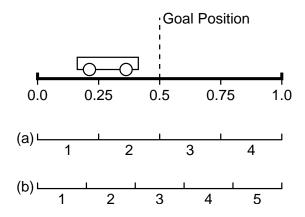
Figure 2.2: An example of poor state discretization.
