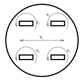
Figure B.1: Synchronous drive locomotion system.
