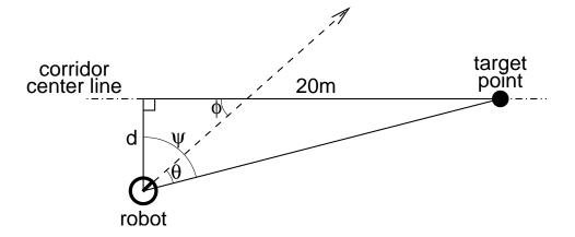
Figure 7.10: Calculation of the angle input feature for the corridor-following task.
