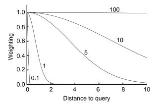
Figure 4.3: Gaussian kernel functions with different bandwidths.
