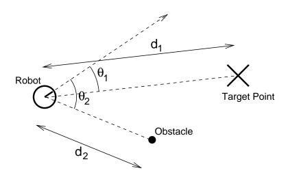
Figure 7.15: The obstacle avoidance task input features.
