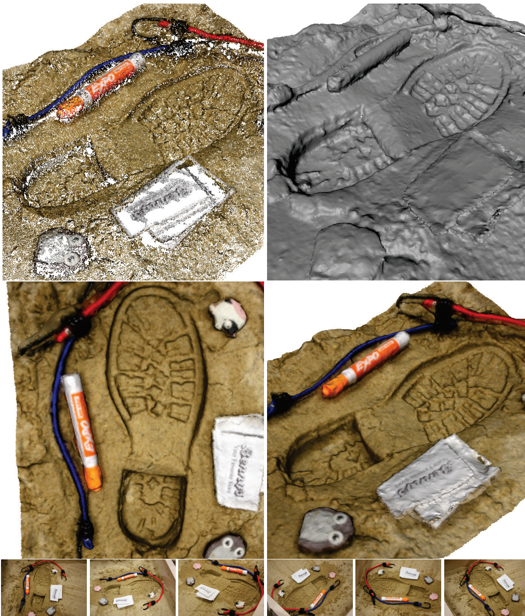
Figure 7: Reconstruction of a shoe print. Top row: the input point cloud (left), and surface geometry (right) reconstructed by the proposed algorithm. Middle row: Two views from surface and color map reconstructed by the proposed algorithm. Bottom row: 6 examples from the set of 11 images that are used for shape acquisition.
