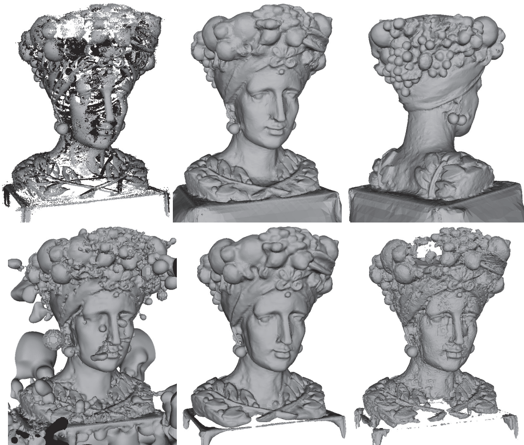
Figure 3: Input point cloud the Chiquita model (top-left), and reconstructions using SSD (top-middle and top-right), MPU (bottom-left), Poisson (bottom-middle), D4 Wavelets (bottom-right) surface reconstruction methods.
