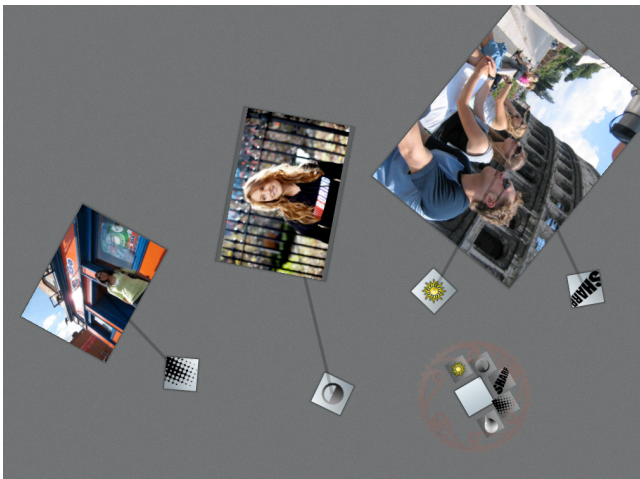
Figure 4: Rearrangeable tokens implemented in “SurfaceShop.” A user adjusts an attribute with a “pinch” gesture on top of its token, the value governed by the distance between his two fingers.
