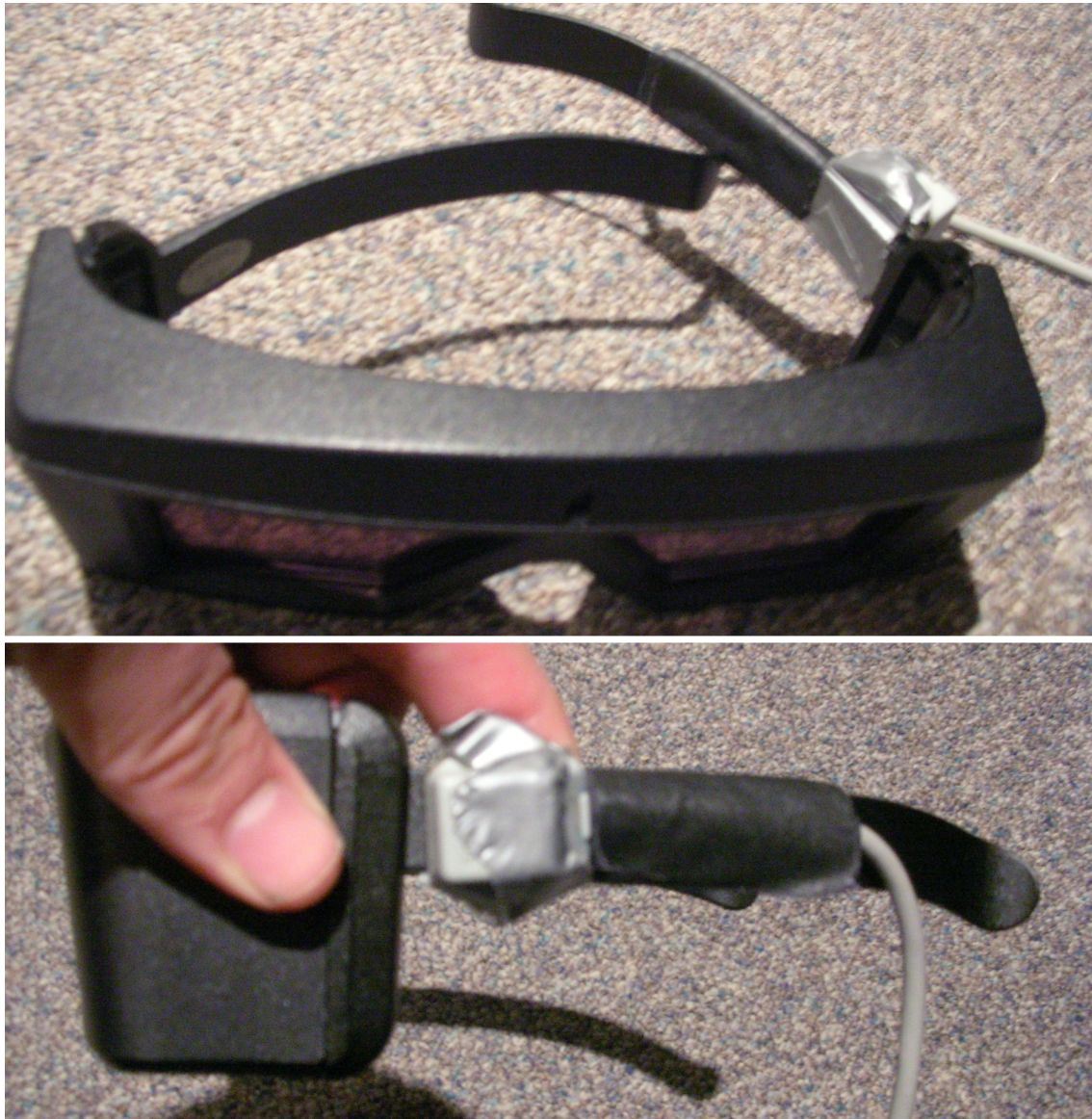
Figure 3.5: Views of the Stereographics shutter glasses with Polhemus tracker attached.
