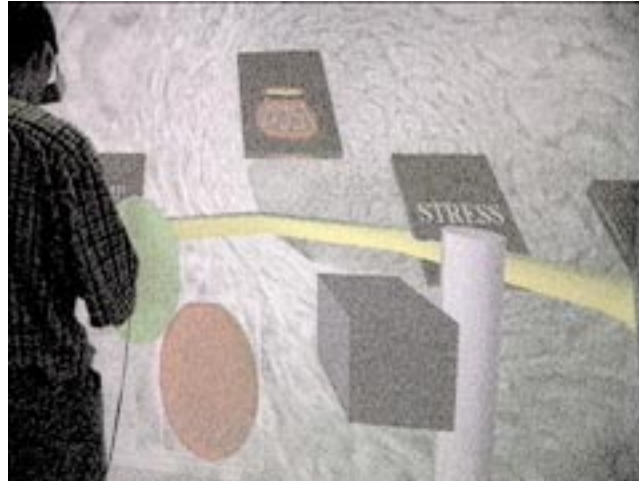
Figure 4.4: When the user looks down a toolbelt appears. Tools include dust, for advecting particles through the flow; a widget for choosing wall coloring; a round alkaseltzer widget for creating a persistent source of advecting particles; an isosurface “microphone” widget (the square cube here); and a streamline and rake widget.
