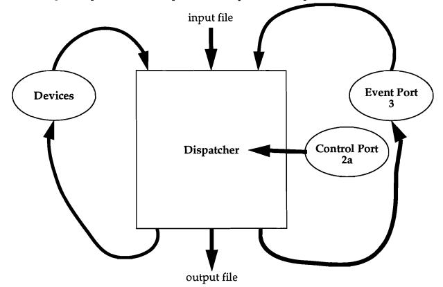
During recording, two or more files are written: *ff* writes the events to an event file, and *audIO* writes one or more audio files, which may later be mixed using the *mix* program to form one audio file. The events are timestamped and recorded immediately before being dispatched so the recording is as close as possible to what the user actually sees.
