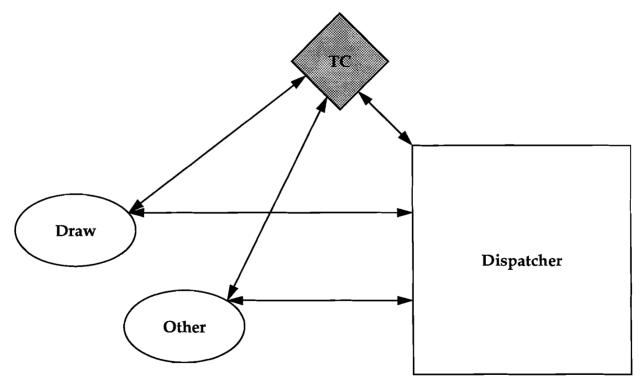
The primary methods declared by the TimeDevice class are jumpTo and playTo. A TimeController will call the jumpTo methods of each device it controls to tell the device to update its screen so that it looks like it did at the given time.
