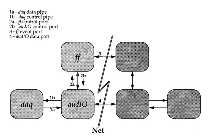
If you are reading the color version of this document, notice that audio data flows along the red lines (1a, 4), control commands along the blue (1b, 2), and events along the magenta line (3). The numbering and colorings of these lines are consistent throughout this paper.
