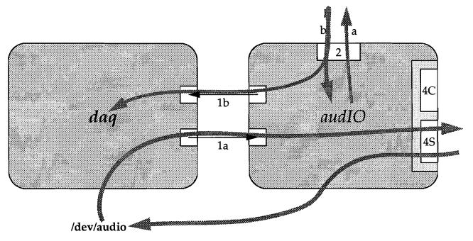
When it starts up, *audIO* creates pipes 1a and 1b and forks. The child process becomes the *daq*. When an *audIO* process connects as a client to another *audIO* process, data will travel through the first process' client socket (4C) to the second process' server socket (4S). Since it is irrelevant which socket is used, these sockets are referred to collectively as the *audIO* data port.
