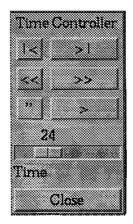
This allows the user to use a graphical user interface to a Time Controller, such as the one depicted above, to jump to any point in time in a recording.
