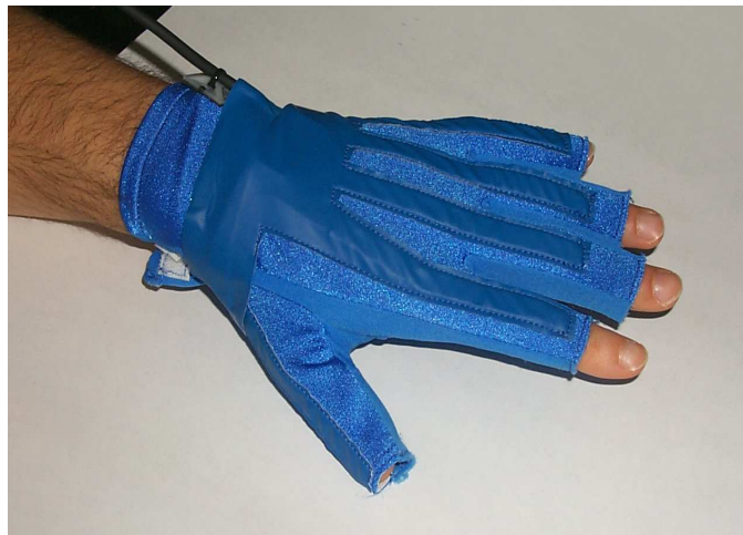
Figure B.3: Nissho Electronic's SuperGlove input device worn by the author. This glove has a minimum of 10 bend sensors and a maximum of 16.
