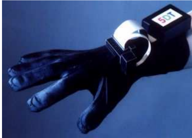
Figure B.2: The 5DT Data Glove developed by Fifth Dimension Technologies. The glove measures seven DOF (from Fifth Dimension Technologies [45]).
