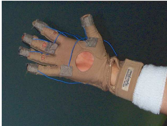
Figure 2.4: The Flex and Pinch input system. The cloth contacts represent the “pinch” part of the device collecting discrete topological data while the glove represents the “flex” part collecting continuous geometrical data. Although a CyberGlove [142] is shown, any bend-sensing glove can be used.
