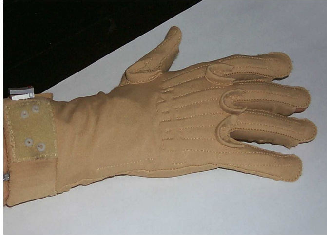
Figure B.6: Virtual Technologies' CyberGlove, worn by the author, which can be equipped with 18 or 22 bend sensors.
