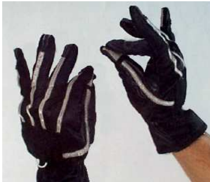
Figure B.4: Fakespace’s Pinch Glove input devices worn by the author. The gloves have electrical contact points that allow users to make “pinch” postures that can be then mapped to a variety of tasks.
