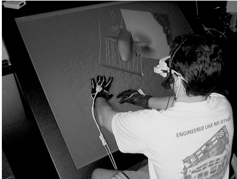
Figure 4.1: A user interacting with a dataset for visualizing a flow field around a space shuttle. The user manipulates the streamlines with his left hand and the shuttle with his right hand while viewing the data in stereo[58].
