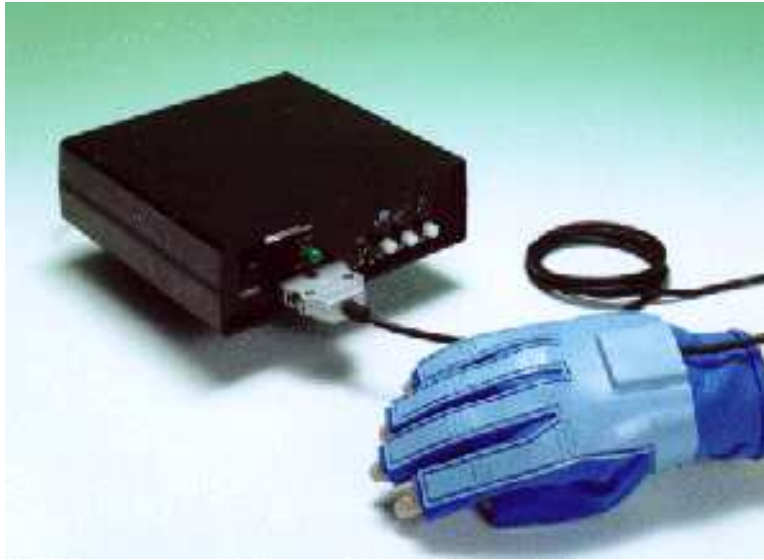
Figure 2.2: Nissho Electronics SuperGlove input device. This glove has a minimum of 10 bend sensors and a maximum of 16 (from Nissho Electronics Corporation[82]).
