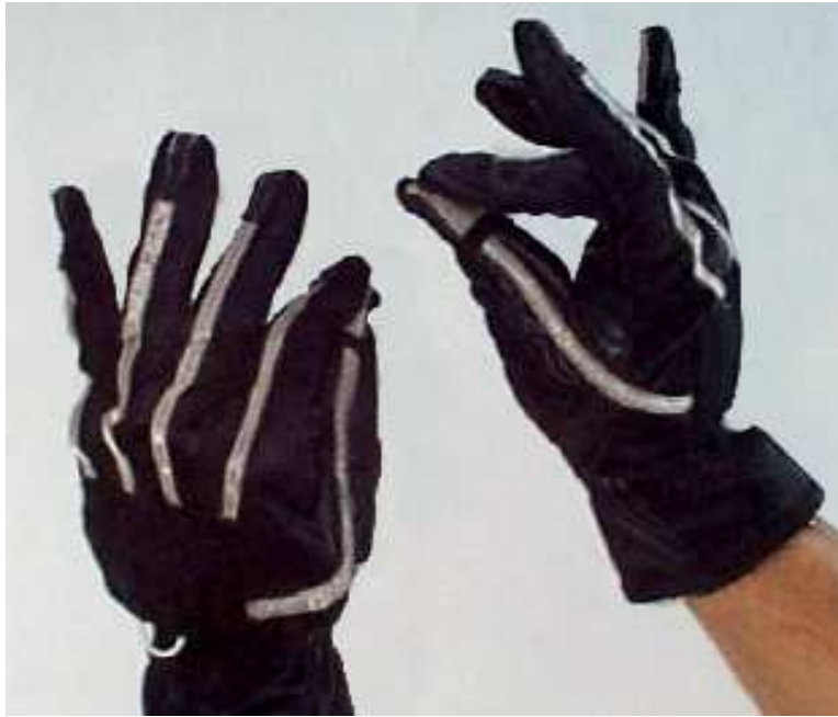
Figure 2.3: FakeSpace’s Pinch™ Glove input devices. The gloves have electrical contact points that allow users to make “pinch” postures that can be then mapped to a variety of tasks.
