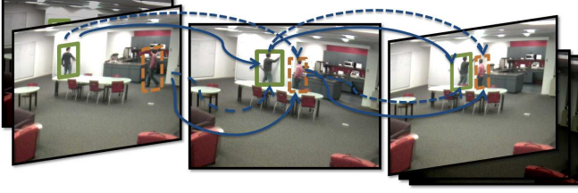
Figure 2: Illustration of Tracking and Data Association using a video captured with our local camera network. Solid lines indicate the correct data associations.
