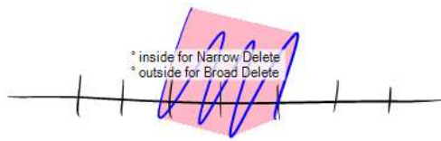
Figure 8: The self-contained gesture for delete. Tapping inside the scribble will delete the contained tick marks. A tap outside the scribble will delete the axis as well. A press and hold inside the scribble makes the stylus act as an interactive eraser until lifted. Anything else leaves the scribble uninterpreted.
