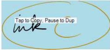
Figure 6: A group of strokes can be copied with a parameterized gesture. First a lasso is drawn around the strokes, then a ‘C’ is drawn inside the lasso. If a tap is drawn the strokes inside the lasso will be copied. If a press-and-hold is done, the strokes will be copied, selected and ready to be interactively dragged.
