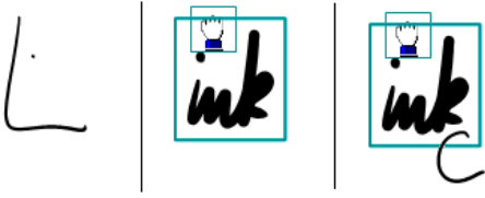
Figure 2: The same action sequence as Figure 1 but done with shortcuts. An L-shaped crop stroke is drawn to specify the lower-left corner of the pasted ink. A tap inside the crop’s hull pastes ink. A ‘C’ overlapping the selection copies the ink. A 200ms pause at the end of C stroke pastes (i.e., duplicates) and drags the copy.
