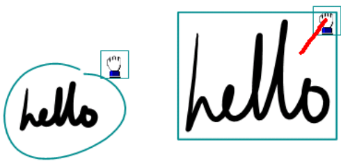
Figure 10: A manipulation widget is placed where the tap was made when the strokes on the left were selected using a Lasso and Tap gesture. By pressing the stylus outside the button and dragging in a straight line through it, the strokes are scaled about the corner opposite the handle. Pressing the stylus inside the button would have dragged the strokes.
