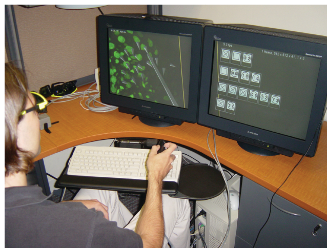
Figure 2. Viewing a cell data set at the Fish Tank system. The user places a marker. We are using two monitors to provide a continuous wider field of view—the control widgets are on the right, and the data set is on the left.
