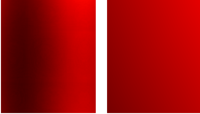
Figure 1: A zoomed-in comparison between the method described here (left image) and a quad drawn only using the corner data points (right image). The important idea is that more detailed information can be shown in the same quad. This left image is drawn with the following data:
