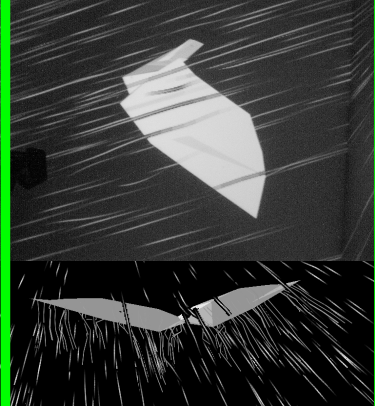
Top, a photo taken in the CAVE shows cylinders representing the paths of particles in the air flow. Bottom, a screenshot in the CAVE shows orange kelp highlighting flow patterns of selected particles.
