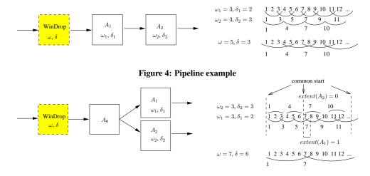
Figure 5: Fan-out example
