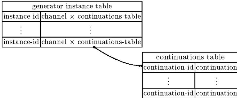
When a thread processes a request to resume its generator’s continuation, it looks up the content generator in one table, and extracts the channel and continuation table for that generator. The server then looks up the desired continuation in this second table and passes it along with the request information and the ports for the current connection.
