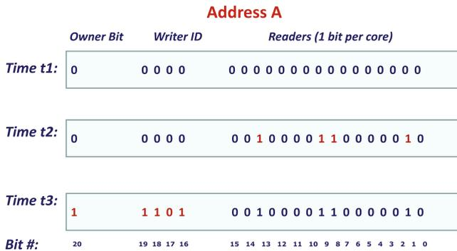
**Fig. 4** Bookkeeping example. At time t1 address location A had not been read or written. By time t2, cores 1, 7, 8, and 13 have read the address. At time t3 core 13 writes the address and generates a conflict. So, core 13 will be aborted and its read flag will be cleared. Since core 13 was also the writer of address location A, the Writer ID bits and the Owner bit will be cleared as well
