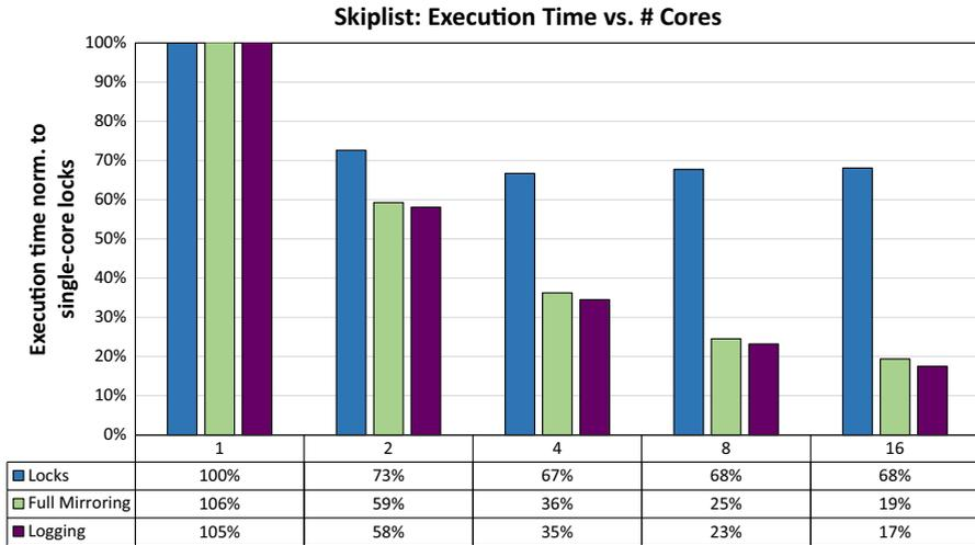
**Fig. 9** Skiplist: performance comparison between locks and transactions for different number of cores
