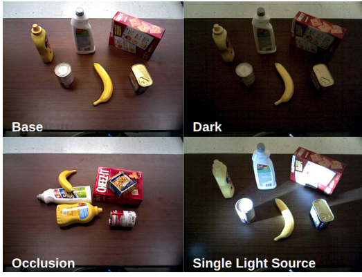
Fig. 4: Testing dataset with YCB objects under adversarial settings. The base-setting data is collected with regular lighting without occlusions. The dark-setting data is collected with lights off in the room. The single lighting data is collected with a flash light. Object poses are the same in previous three settings. Data in three occlusion scenes is collected with the same objects randomly stacked.
