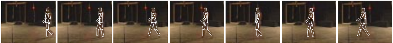
Figure 7. Tracking of a walking subject. The 7 images are frame 0, 5, 10, 15, 20, 25 and 30 of the sequence. Overlaid on the images are the weighted means of the posterior probability distribution.
