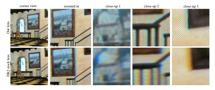
Fig. 18: This is a view of the Oculus Rift display as seen by our lens (top row) and the Oculus Rift lens (bottom row). The Oculus lens has significant residual chromatic aberration, even after the software pre-processing that Oculus performs to correct chromatic aberration. For our lens chromatic aberration is so small that no software correction is needed. Other aberrations are also much smaller. Best viewed electronically.
