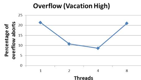
**Figure 6.** Example of overflow due to hyper-threading (vacation high benchmark).
