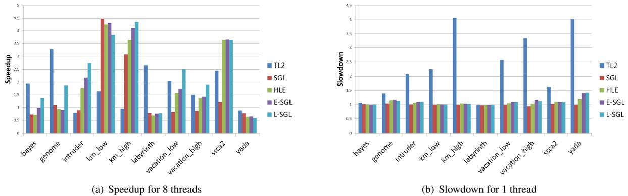
Figure 9. Speedup for 8 threads and slowdown at 1 thread, compared to sequential.
