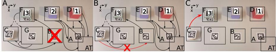
Fig. 7: Additional constraints for: (A) Unrealizable Specification 1 (the block cannot move into location B,  $\square \neg \bigcirc (\sigma_0 \wedge \sigma_{15})$ ), (B) Unrealizable Specification 2 (skill  $a_{c \rightarrow b}$  is not allowed). (C) The skill,  $a_{c \rightarrow f}$ , used to repair Unrealizable Specifications 1-4.
