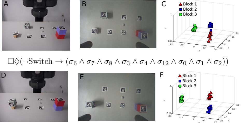
Fig. 5: (A,B,C) Where the blocks should be when  $\text{switch} = \top$ . (D,E,F) Where the blocks should be when  $\text{switch} = \perp$ . (A,D) As seen by an observer. (B,E) As seen by the Baxter's left hand camera. (C,F) As represented by sampling 10 points from the grounding sets of the  $\top$  symbols. Above each row is the liveness formula.
