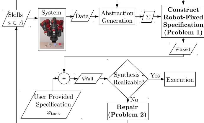
Fig. 2: Framework for automatically encoding robot capabilities, executing tasks, and repairing unrealizable tasks. Novel contributions are in bold.
