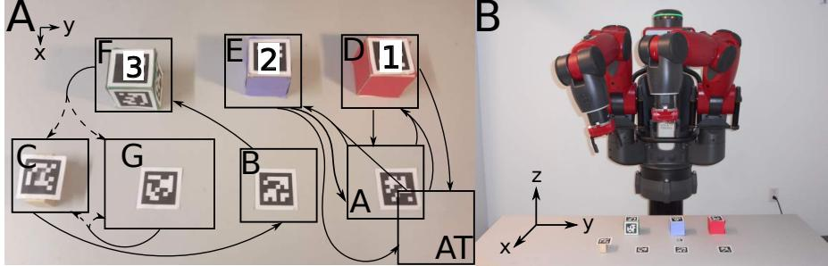
Fig. 3: (A) Example 2: Block manipulation domain. The arrows show the skills given to the robots to move blocks between lettered locations. Dashed arrows represent skills with nondeterministic outcomes. One skill takes blocks from A and AT to D and another from A and AT to E. (B) Initial setup of the Baxter robot and blocks.
