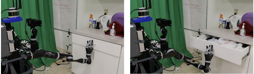
Figure 7: **Novel object manipulation.** A MOVO robot manipulating a novel drawer using a kinematic model estimated from a single depth image.
