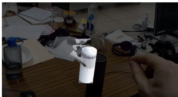
b) A user repositioning the 3D mesh of a robot end-effector to ground the grasp pose relative to the item.
