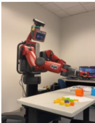
Figure 1: The Baxter robot used for the TagUp system.
