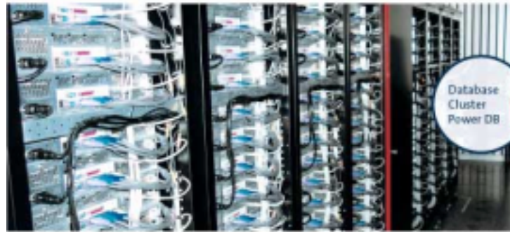
Figure 3 Physical View on the database cluster of 128 DBMS nodes
