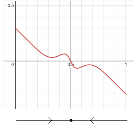
(b) Graph of \frac{\partial l}{\partial t} with c = 0.7 and corresponding phase portrait. l on x axis, \frac{\partial l}{\partial t} on y-axis
