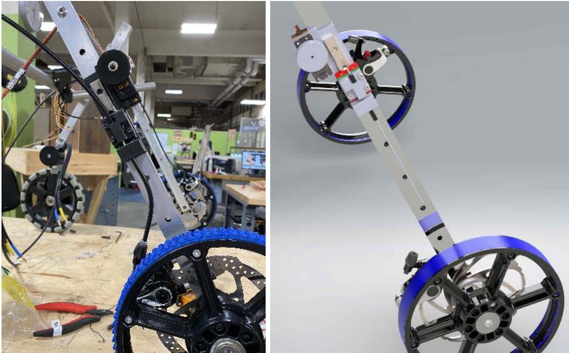
Figure 2.15: Inline braking system in Mark III
