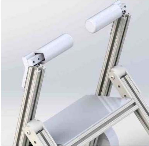
Figure 2.7: Mark 0 Horizontal Load Cells
