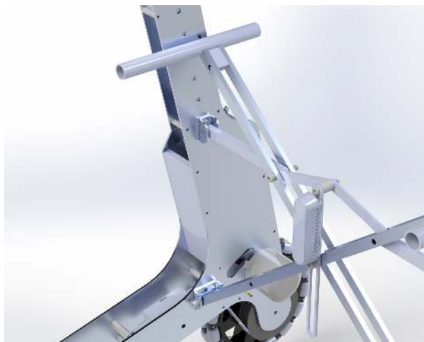
Figure 2.25: Mark IV folding structure
