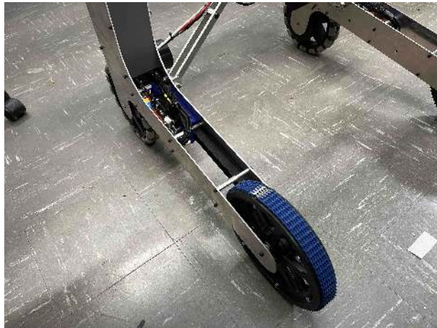
Figure 2.20: Mark IV belt with tensioning
