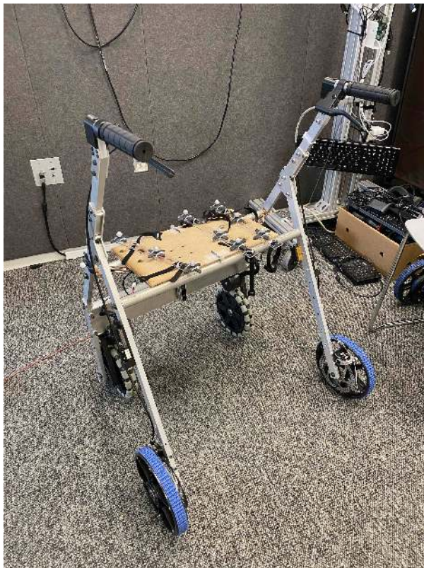
Figure 4.2: Custom MOCAP markers were made with the goal of tracking the location and angle of users' thighs and upper body
