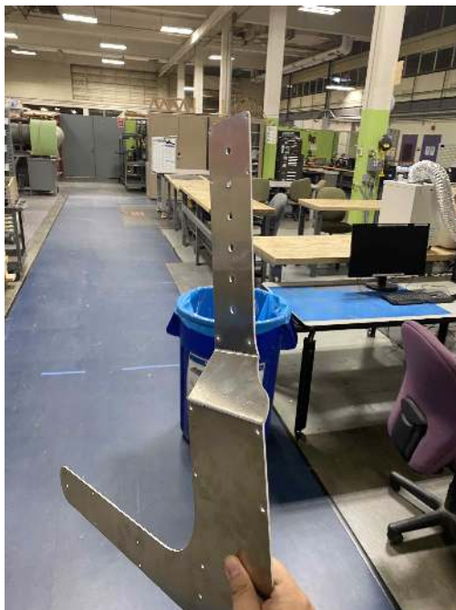
Figure 2.30: Folded sheet metal for Mark IV exterior
