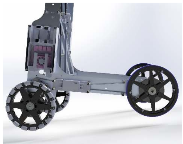
Figure 2.19: Mark IV motor-belt all wheel drive assembly with belt tensioning
