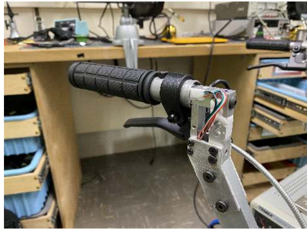
Figure 2.10: Dual Load Cell Handle Design
