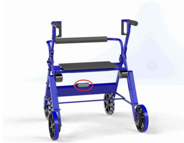
Figure 2.12: Mark II RealSense placement Figure 2.13: Mark III RealSense Placement
