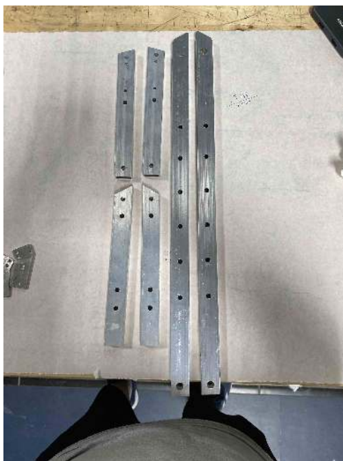
Figure 2.28: Mark III's prime structure extrusions
