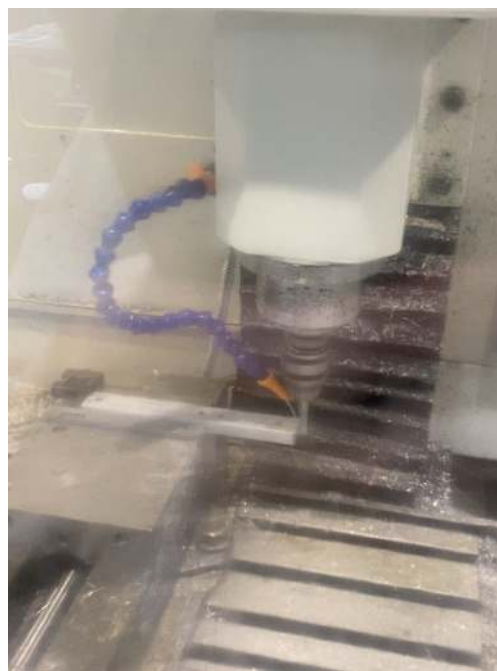
Figure 2.29: Using the Tormach to machine the Mark III legs
