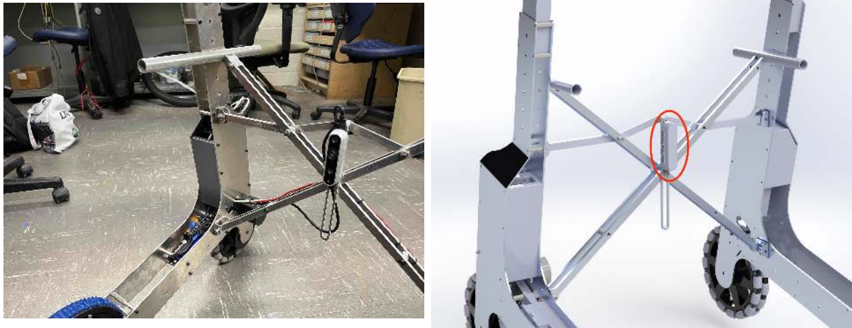
Figure 2.14: Mark IV RealSense Placement
