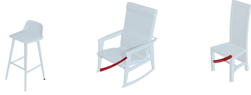
Figure 2. Examples of foot, rocker, and bar stretcher renderings from PartNet. The fixed viewpoint limits visibility of small or occluded parts.
