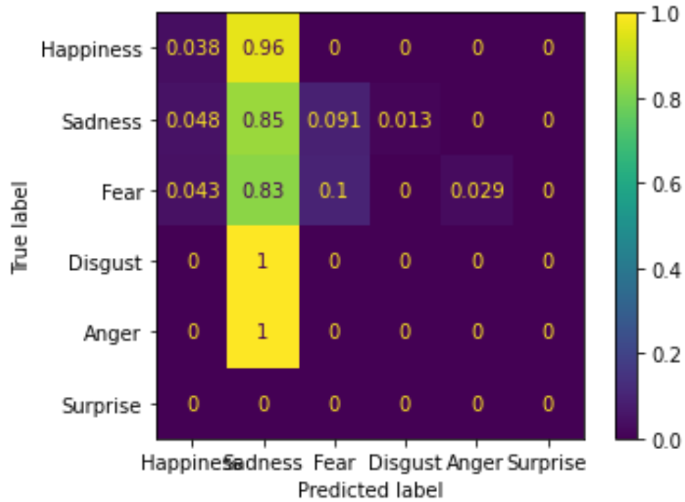
FIGURE 4. Confusion matrix of original ResNet-50 outputs with SMOTE applied on dataset (for comparison).
