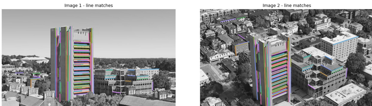
Figure 2: LightGlueStick matches on a Google Earth render pair with 30^\circ of angular separation. Inlier correspondences are dense and structurally correct across building facades and roof edges.
