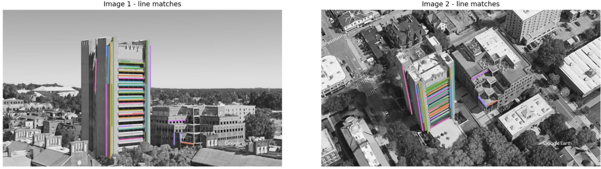
Figure 3: LightGlueStick matches at 60^\circ . Inlier count drops and spurious matches appear, though prominent structural lines are still recovered.
