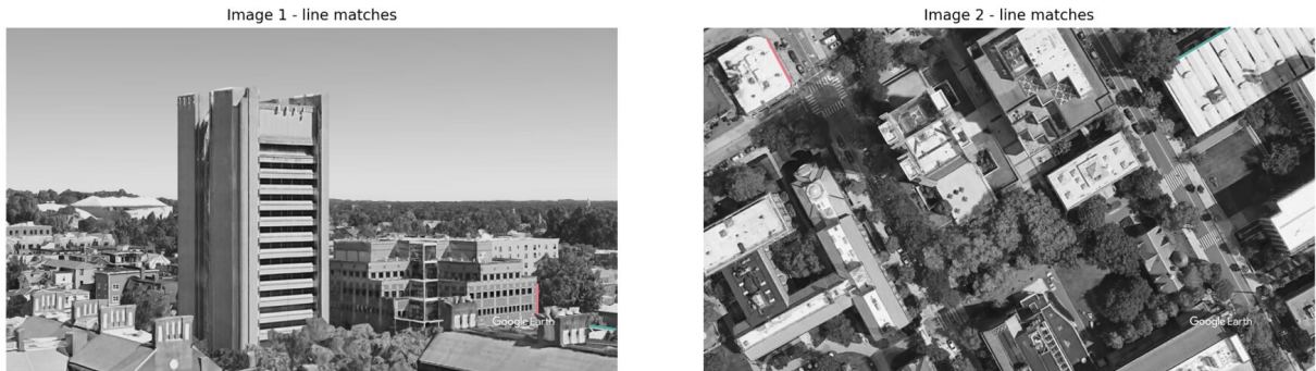
Figure 4: LightGlueStick matches at 90^\circ . The recovered correspondences bear no structural relationship to the actual scene geometry; matching has collapsed.
