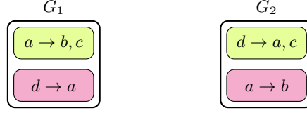
Fig. 4: Node a is in the tail of one edge and the head of the other hyperedge in each dihypergraph. The corresponding MC is not irreducible.
