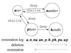
Figure 5: Deletion and restoration ordering in DELF when object  $\boldsymbol{u}$  is deleted. Two-letter log entries denote edges from/to the corresponding objects. Objects are deleted before and restored after their outbound edges.
