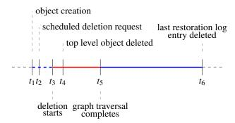
Figure 2: Timeline of a deletion in DELF. The time period between the start of a deletion  $(t_3)$ , the end of graph traversal  $(t_5)$ , and restoration logs deletion  $(t_6)$  should match the service provider's deletion policy.
