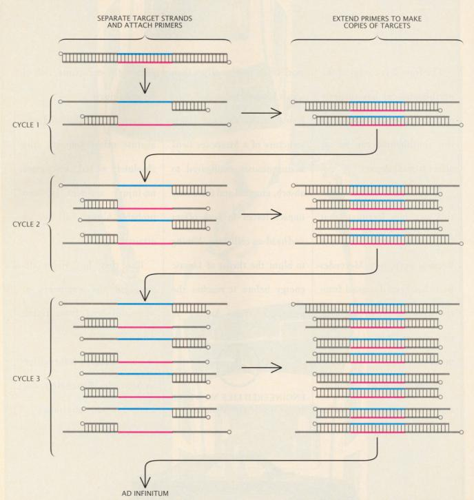
POLYMERASE CHAIN REACTION is a cyclic process; with each cycle, the number of DNA targets doubles. The strands in each targeted DNA duplex are separated by heating and then cooled
