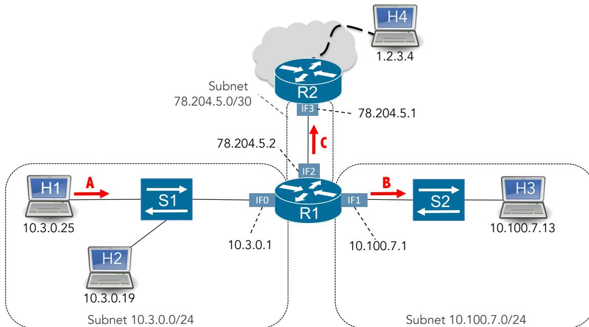
a) First, H1 sends an IP packet to H3. (Assume that this sends an ARP request, which happens successfully.) For the IP packet, write the source and destination addresses in both the L2 (Ethernet) and L3 (IP) header when it is crossing the link labeled A in the figure. For MAC addresses, you can use names based on the name of the host or router interface, eg. MAC\_H1 for H1, MAC\_IF1 for R1's IF1, etc.
