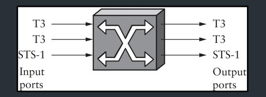
Switches must be able to, given a packet, determine the outgoing port
