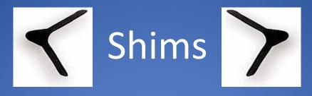
It is often possible to open a padlock by slipping shims in between the shackle and the lock's casing
