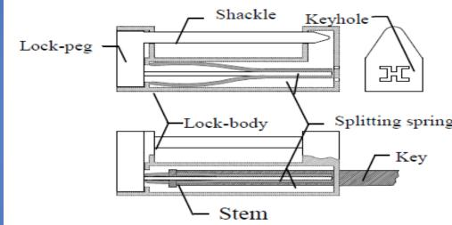
•For opening, key is inserted and its head squeezes the opening springs so that the sliding bolt can exit from lock-body.
