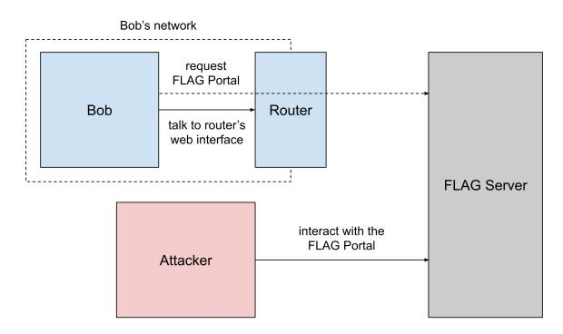
Figure 1: Network configuration for Bob's Router.
