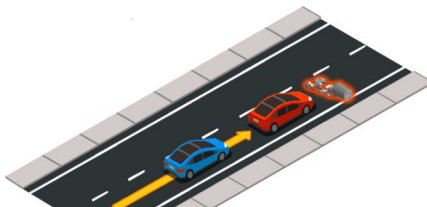
Traffic Scenario 02: Longitudinal control after leading vehicle's brake
