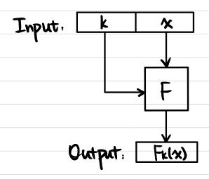
If F is model as an "ideal cipher", them Davies-Meyer Construction is Collision-resistent.
