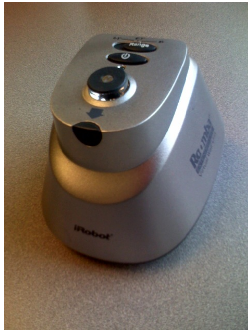
Figure 1: An iRobot Virtual Wall device emits an IR signal that can be received by the SmURV and provided to your client by Player’s IR proxy.
