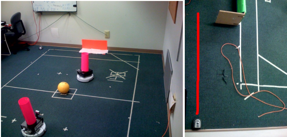
Figure 2: Snapshot of the “FC 148” robot soccer field surrounded by virtual infrared (roughly marked in red) and real walls. Your robot should properly react to both types of obstacles and other robots (with pink fiducials).
